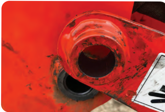
The lift pin on my Kubota backhoe broke while digging. (Photo by Blaine Howerton)
